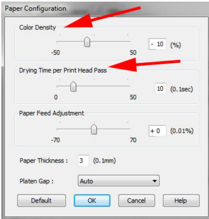
Above is an example of the Paper Configuration controls of an Epson 3880. Most wide format Epson printers have this same setup.
