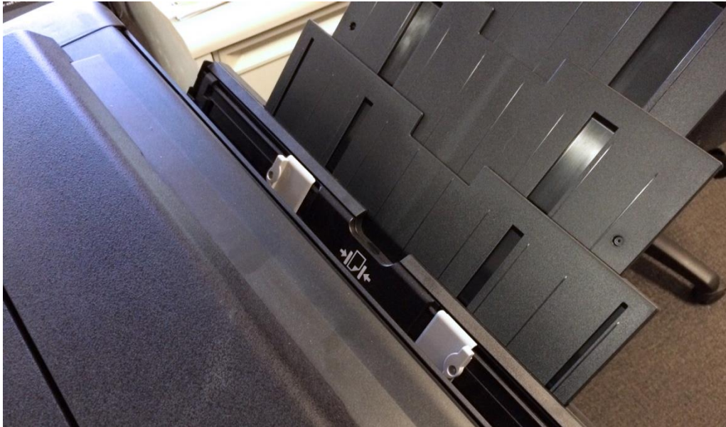
Pictured Above - the Canon PRO-1000 rear single sheet feed path.
